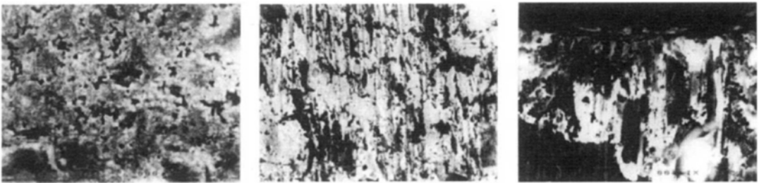
(a) Unworn appearance (b) Worn appearance of rake face (c) Worn appearance of flank face
